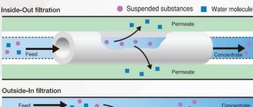
A high cross - flow velocity over the membrane surface prevents membrane fouling. This makes inside - out filtration suitable for concentration and purification of highly concentrated solutions.
